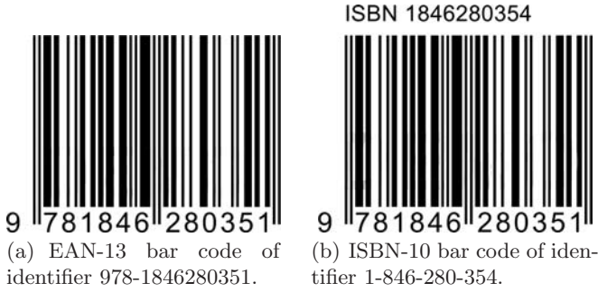
Fig. 5.1. Two bar codes encoding numbers that refer to the same object under two different identifier systems. The object identified is the book of reference [100].
