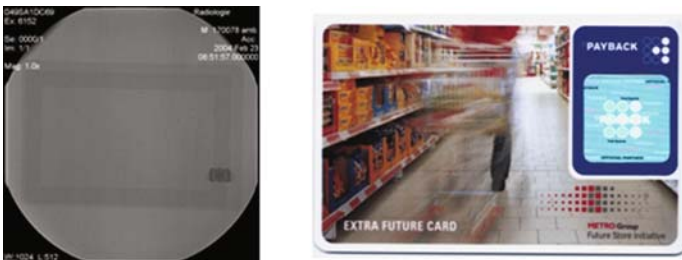
Fig. 9.1. Loyalty card issued to the visitors of the Metro Supermarket of the Future and an x-ray image of the card showing the embedded tag. Photos by Peter Ehrentraut, FoeBuD.
