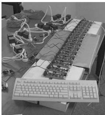
Fig. 9.3. Cracking the encryption of the TI DST tag used in the Mobile Speedpass system using low-cost FPGA hardware.
