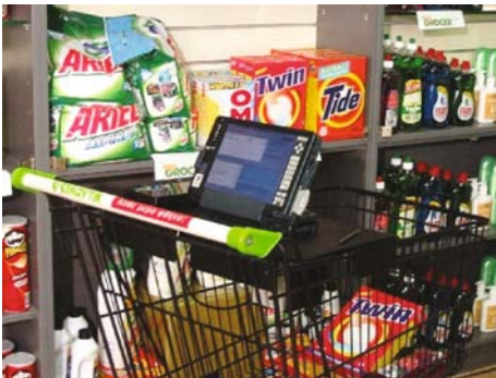
Fig. 10.3. Prototype shopping cart implementation: shopping cart with tablet PC, wireless network, and RFID reader (left). User interface: login screen, shopping options, including shopping cart content monitor, shopping list, total shopping cart content cost, offers and personalized promotions, additional product information, and finally fast checkout (right).
