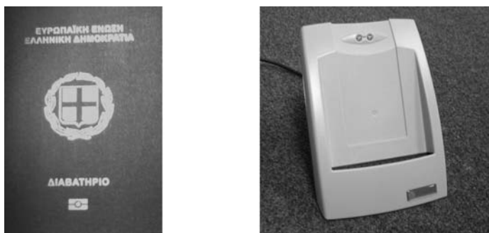
Fig. 2.1. A Greek e-passport and an associated reader. Note the mark at the bottom of the front cover of the passport indicating that it is MRTD compliant. The Greek MRTD system has been developed by Arcontia in collaboration with ACG.
