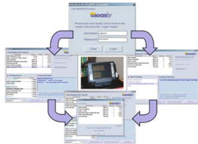
Fig. 10.3. Prototype shopping cart implementation: shopping cart with tablet PC, wireless network, and RFID reader (left). User interface: login screen, shopping options, including shopping cart content monitor, shopping list, total shopping cart content cost, offers and personalized promotions, additional product information, and finally fast checkout (right).
