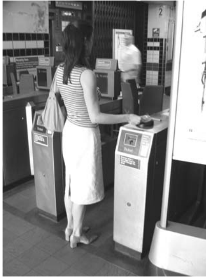
Fig. 2.4. Entering The Tube using the Oyster card. Note the placement of the Oyster on the special indicator, which ensures accurate reading and the displays embedded on top of the gates, which provide visual and sound feedback.
