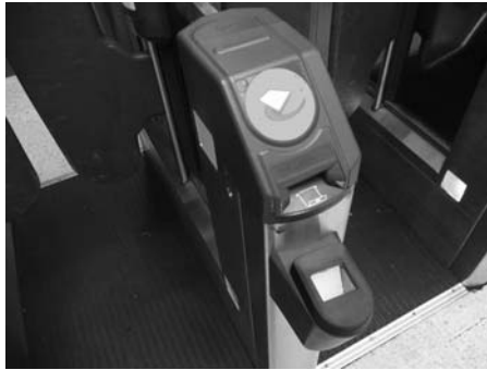
Fig. 2.3. An RFID ticket validator at the gates of the London Underground network.
