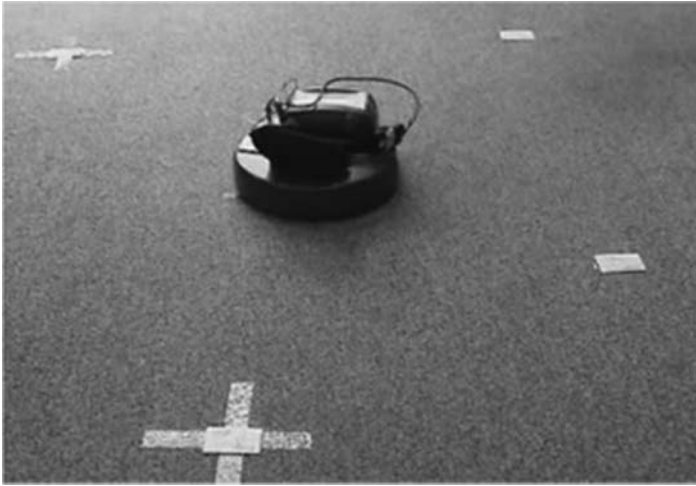
Fig. 10.2. A mobile sensor node (the Roomba cleaner) with a surrogate device capable of sensing its location from RFID tags.
